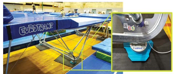
Figure 1: Measurement of flight time and landing position, using an all-in-one measurement system (HDTS EU-7100).
