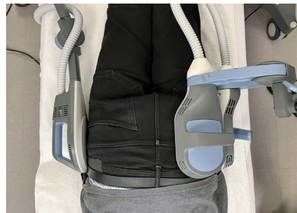
Figure 3: Experimental setup for comparing subjective perceptions during hip stimulation using single-coil (left limb) and double-coil (right limb) configurations.
